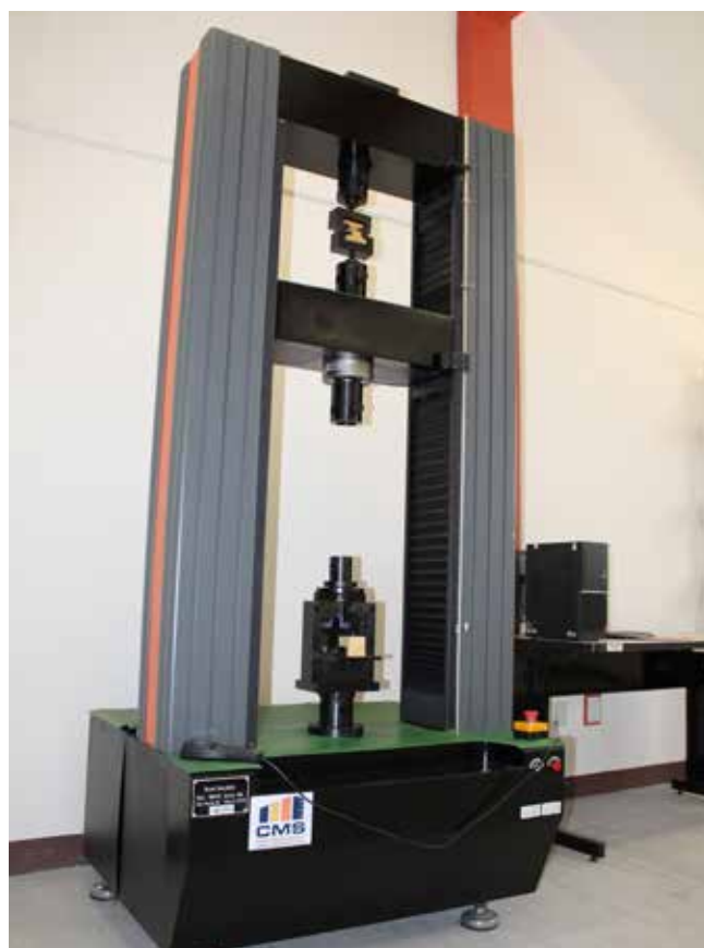
Universal CMS Metrology machine for wood mechanics testing. UNSIJ. Ixtlan de Juárez.
