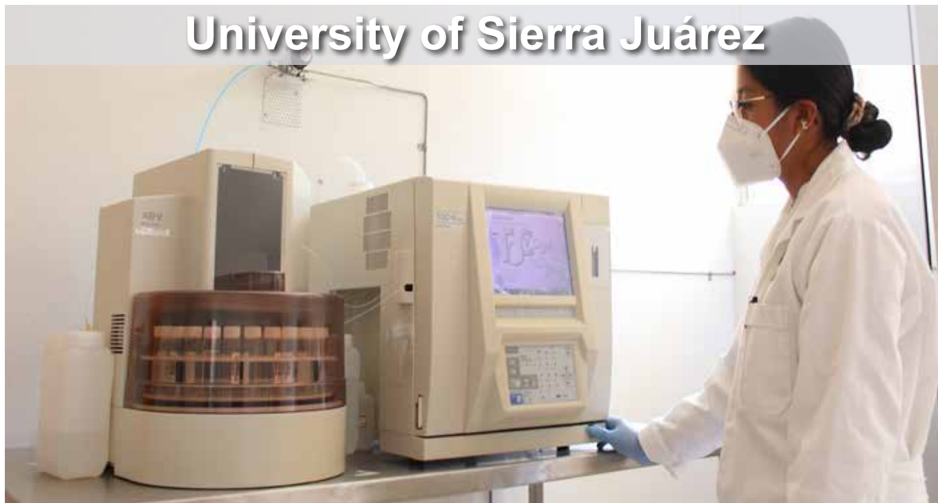
Total carbon analyzer. Earth Sciences Laboratory. UNSIJ. Ixtlan de Juárez.
