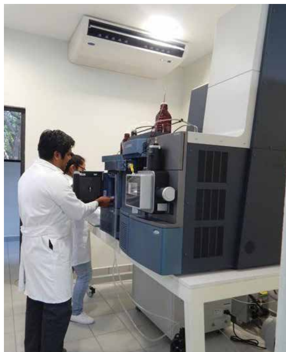
Ultra high pressure liquid chromatograph coupled to a mass spectrometer. Biotechnology Laboratory. UTM. Huajuapán de León.
